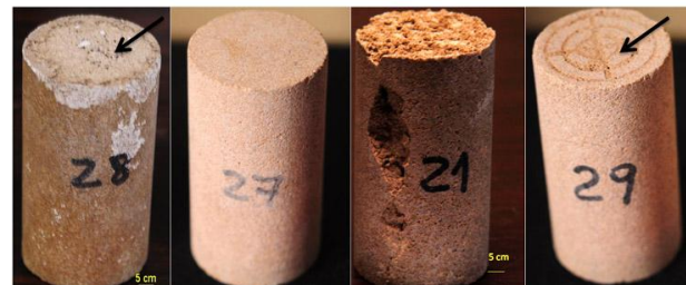
Figure 1: Indiana carbonate core samples used in the acidizing procedure performed with EDTA.
